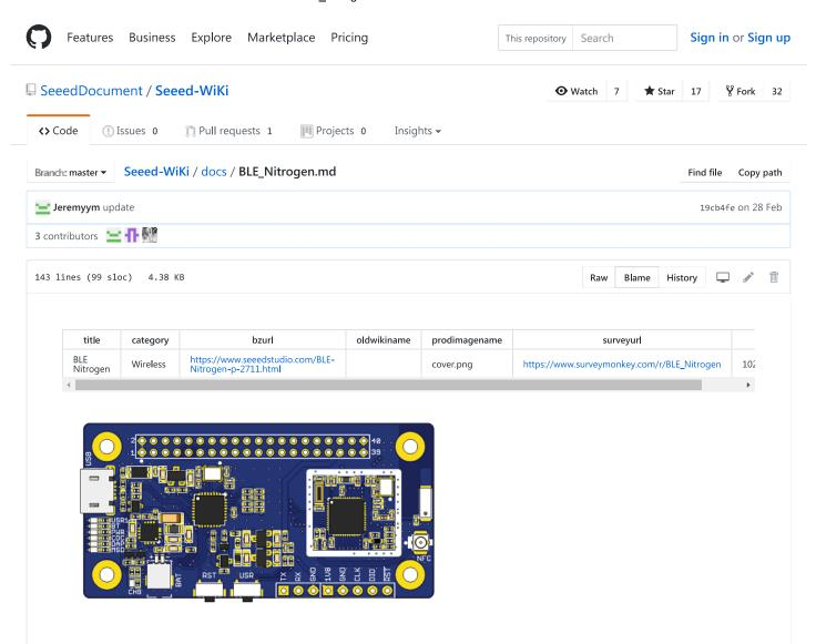
Zephyr applications use the nrf52\_nitrogen configuration to run on the nRF52 Nitrogen hardware. It provides support for the Nordic Semiconductor nRF52832 ARM Cortex-M4F CPU and the following devices:
